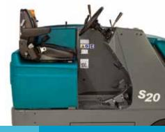
a 1,575 mm sweeping path that shortens cleaning time by adding optional dual side brushes and a high-capacity debris hopper. Increase safety and effective operation in the most severe environments with an optional overhead guard or the optional soft side cab that can be installed or removed in minutes to adjust for changing weather conditions.
